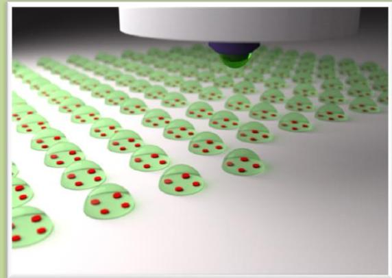
After dispensing, a droplet evaporates, leaving solute on the surface. The size of solute can be controlled by precisely tuning the properties of the surface.
