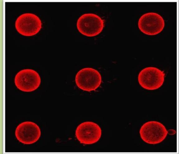
Up to 10 different solutions can be deposited, creating a gradient or an array chip
