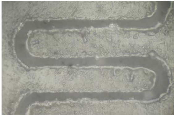
Figure 18. Trenches at high fluence (acetal copolymer, 266 nm, 41 J/cm 2 ).
